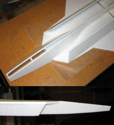
6. Glue the forward fuselage lower assembly in place on the front of the wing. Make sure the aft end of the forward fuselage mates with the forward edge of the centerline support piece. Also make sure the curvature is smooth as the angled forward fuselage sides twist to meet the vertical centerline support. Some trimming and additional heat-forming will likely be required to get a smooth curve here.
